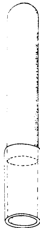
TOOLS. Figure 2. A reconstructed bow-driven drill shaft, fitted with its copper tube. (Courtesy Denys A. Stocks)
