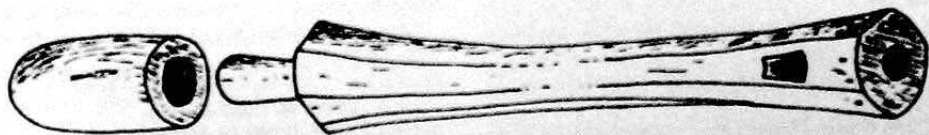
TOOLS. Figure 1. Kahun bow-driven drill stock, with its wooden drill cap. A tool can be removed by pushing a short stick into the ejection hole. (Drawn from Manchester Museum Catalogue number 23. Courtesy Denys A. Stocks)
