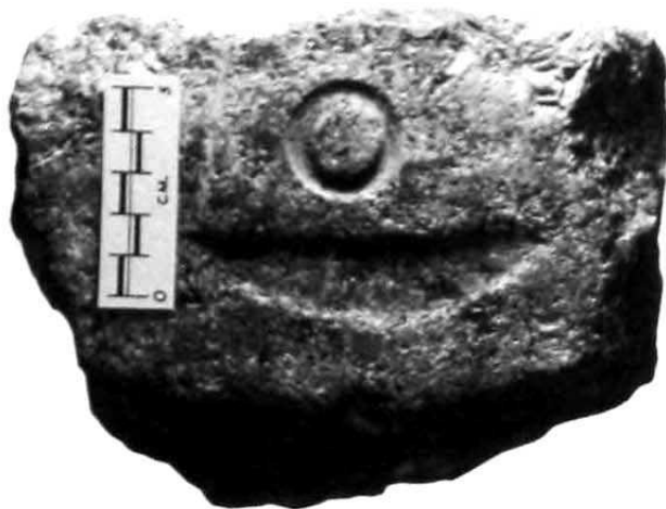
STONEMWORKING. Figure 3. The biliteral sign nb cut into granite by test flint punches and chisels. The sign was polished by sandstone grinders and drilling powders of the waste material.
